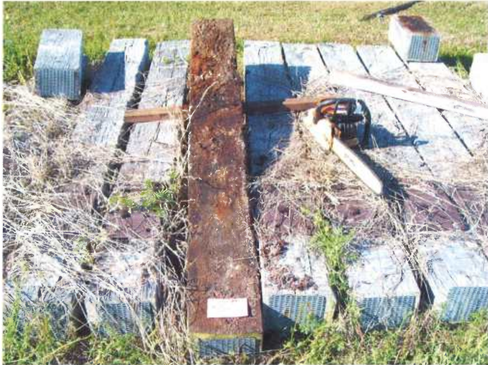
Figure 17 - Tie #87 (Lonza/red oak) decay and trace termite damage.
