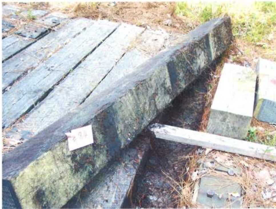
Figure 15 - Tie #84 (Boatright/red oak/borate/creosote 5pcf).
