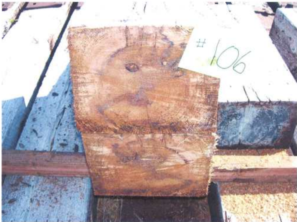
Figure 22 - Tie #106 (Nisus/red oak/borate/oil B) with knots in cross-section.
