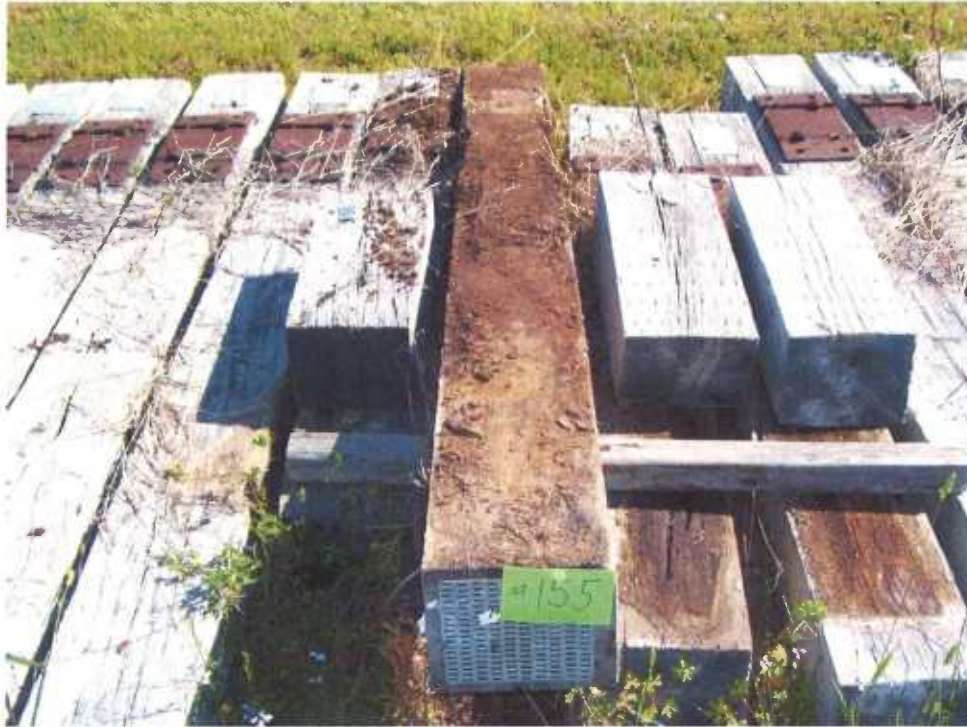
Figure 31 - Tie #155 (Nisus/white oak/borate) with light decay on bottom.
