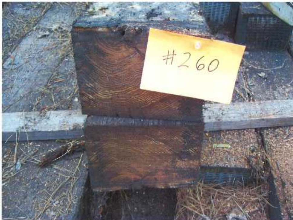
Figure 58 - Tie #260 (Koppers/red oak/creosote petroleum).
