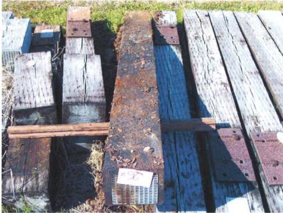
Figure 19 - Tie #96 (Nisus/red oak/borate/oil A).
