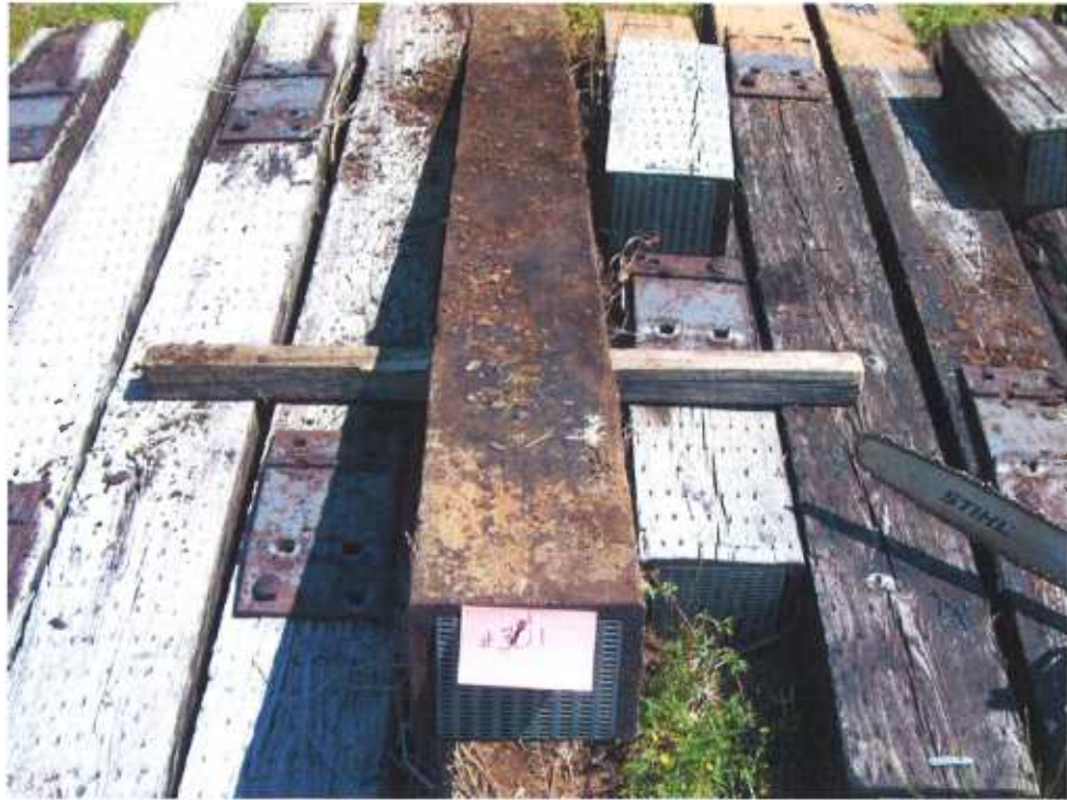
Figure 59 - Tie #301 (Koppers/red oak/creosote petroleum).
