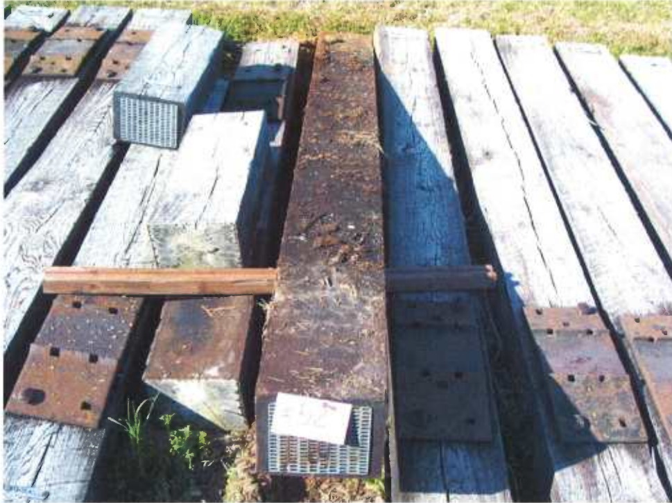
Figure 11 - Tie #52 (Boatright/white oak/creosote to refusal) light decay on bottom.
