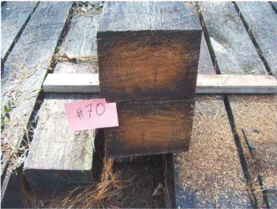
Figure 14 - Tie#70 (Boatright/red oak/creosote 5pcf).
