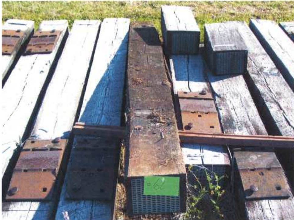
Figure 13 - Tie #62 (Boatright/white oak/borate/creosote to refusal).
