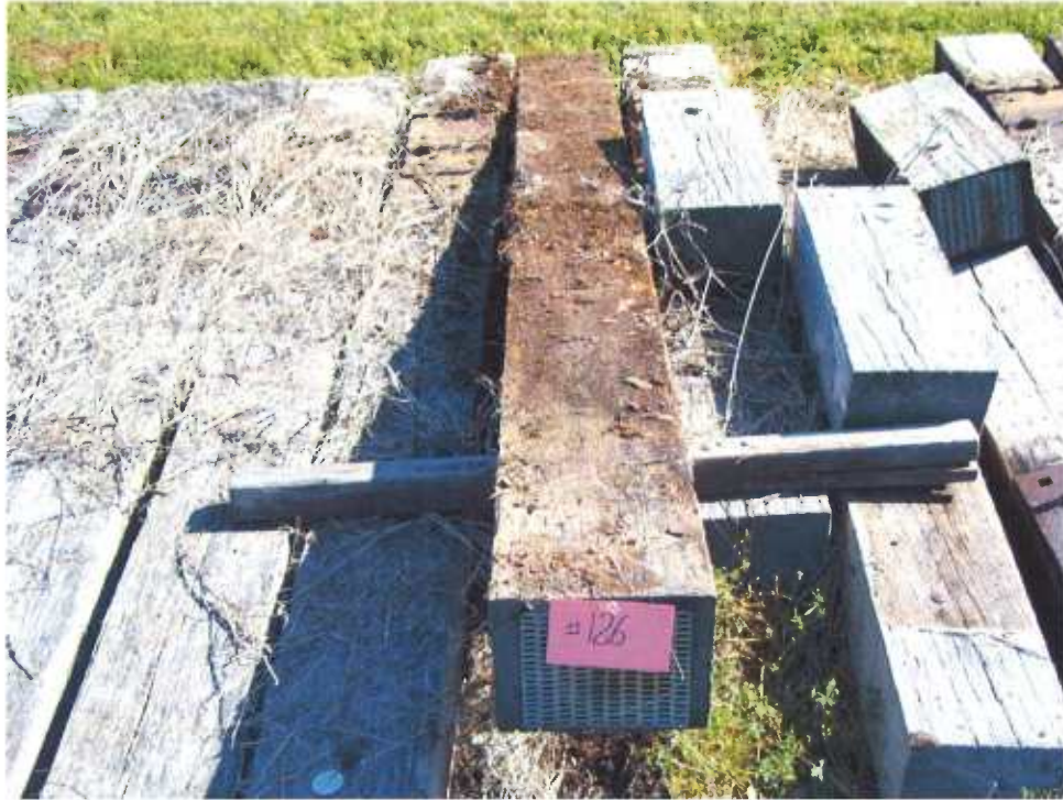
Figure 25 - Tie #126 (Nisus/red oak/borate) with decay on bottom.
