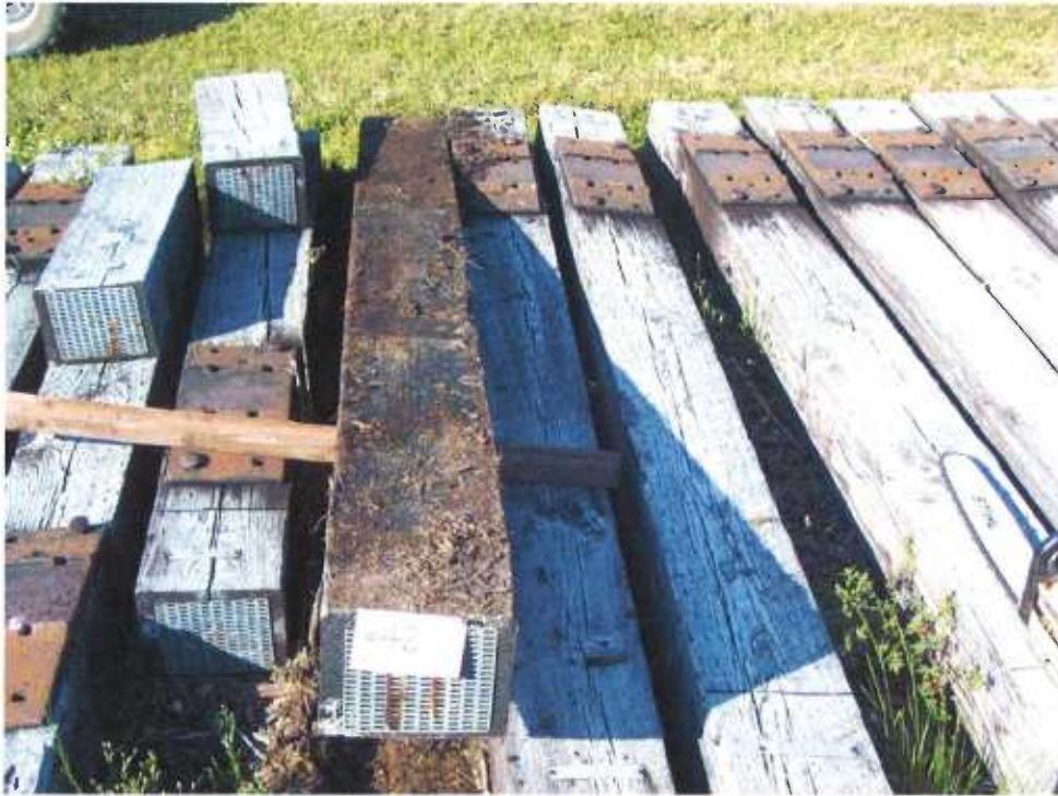
Figure 9 - Tie #42 (Boatright/red oak/borate/creosote 5pcf).
