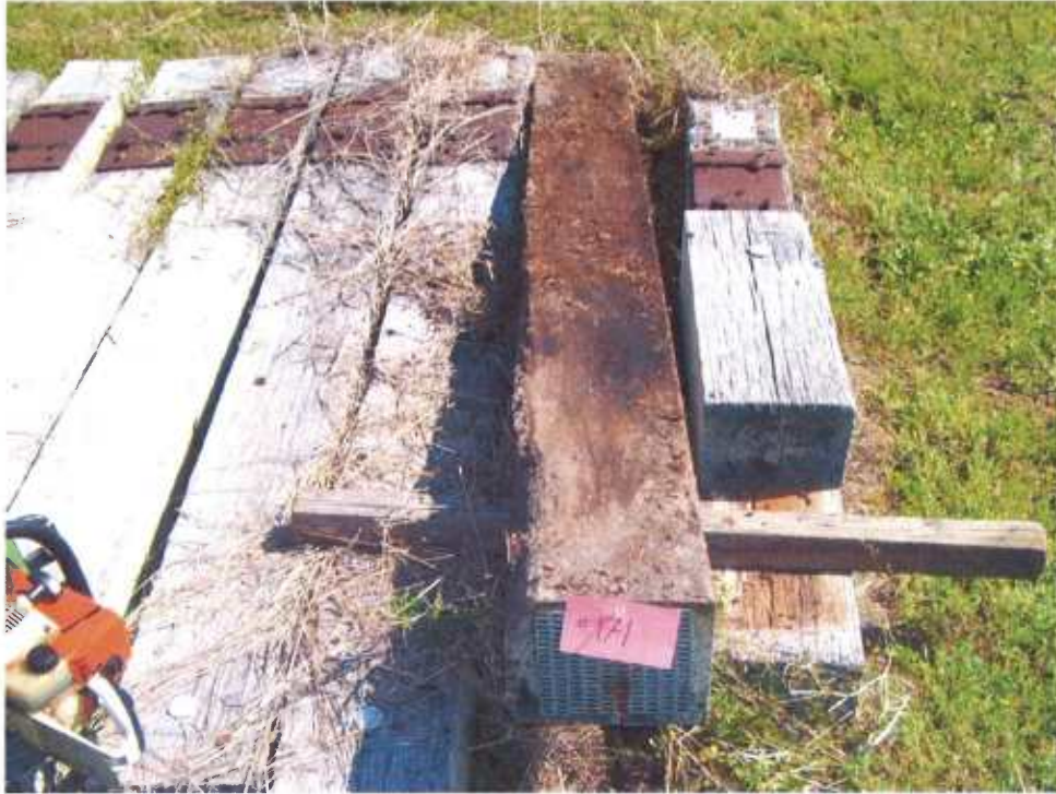
Figure 37 - Tie #171 (Lonza/red oak) light decay on bottom and side.
