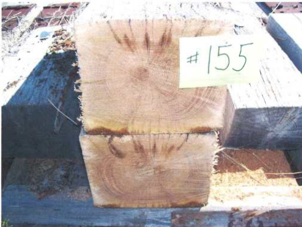
Figure 32 - Tie #155 (Nisus/white oak/borate) with decay on bottom.
