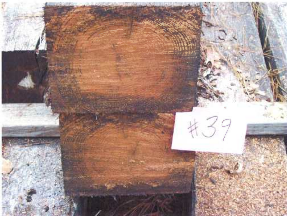
Figure 8 - Tie #39 (Boatright/red oak/borate/creosote 7pcf).
