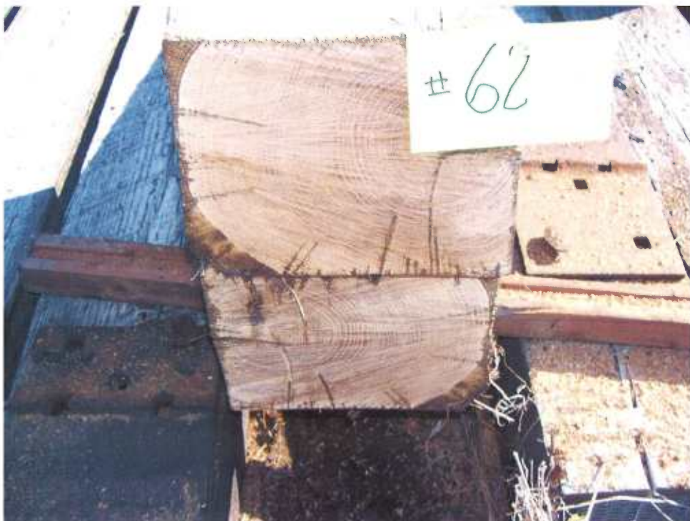
Figure 14 - Tie #62 (Boatright/white oak/borate/creosote to refusal).
