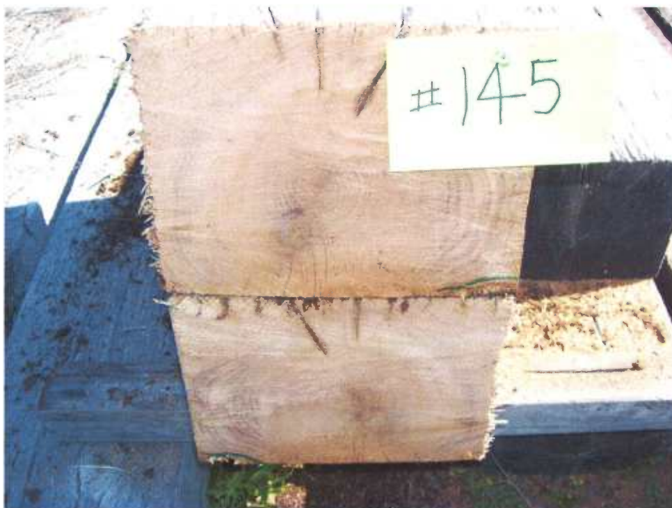
Figure 30 - Tie #145 (Lonza/white oak) with decayed area marked.
