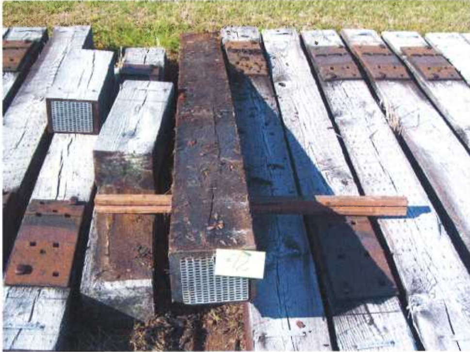
Figure 15 - Tie #72 (Boatright/red oak/borate/creosote 7pcf).
